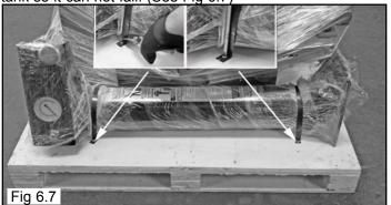
6. Remove the two front and rear bolts and nuts fastening the tire changer to the pallet. (See Fig 6.8 - 6.9)
