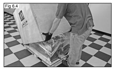
4. Carefully cut the Tire Changer free of the plastic wrapping securing it to the Tire Changer base. Do not unwrap the Assist Tower and Tower Tank at this time. The wrapping helps keep the Swing arms from moving during lifting and assembly. (See Fig 6.5 - 6.6)
