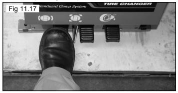
11. Hold the Bead Lifting Tool down until the upper bead is solidly above the rim. Continue rotating the wheel clockwise until the upper bead is completely demounted. (See Fig 11.18 - 11.20)
