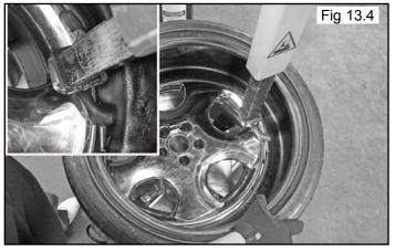
5. Manually push the tire down into the drop center of the wheel directly across from the Mount/ Demount Head to reduce the tensional force on the bead. Depress the Table Top Pedal and rotate the wheel to begin mounting the lower bead. Rotate the Table Top until the lower bead is fully mounted. (See Fig 13.5 - 13.6)
