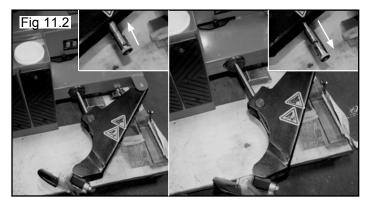
6. Position the bead breaker blade against the tire next to, but not on, the rim or the sidewall of the tire. Press the breaker pedal to actuate the blade and loosen the bead. It may be necessary to loosen the bead in multiple locations around the tire. Use extra care in positioning the bead breaker blade on larger wheels/tires, and on alloy wheels. (See Fig. 11.3)
