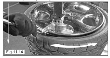
8. Insert the smooth curved end of Bead Lifting Tool over the right end knob of the mount/demount head and below the top bead of the tire. (See Fig 11.15)
