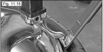
9. Push the Bead Lifting Tool down toward the wheel to lift the tire bead up and over the tab of the demount head. Hold the Bead Lifting Tool in this position. (See Fig 11.16)
