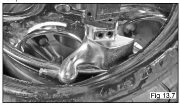
7. With the Bead Lifting Tool, press down on the tire to hold the upper bead in the drop center. (See Fig. 13.8)
