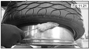
13. Lift and hold the tire so it is positioned with the lower bead in the drop-center portion of the wheel.
