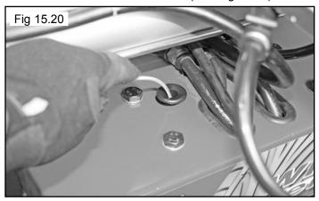
3. Remove the wire and check the level of the Transmission fluid. The oil should cover no more than 1" ( 25 mm) of the wire.
