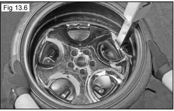
6. For the top bead, rotate the Table Top until the valve stem is at the 3 o'clock position in relation to the Mount/ Demount Head. Lift the upper bead above the right side of the Mount/ Demount Head and below the knob. (See Fig 13.7)
