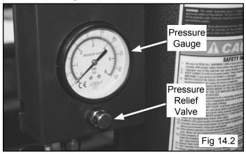
**Position Two** - Tire Inflation - With the Inflation Hose attached to the tire valve and the pedal depressed, line pressure is allowed to flow through the valve and into the tire for inflation. Tire pressure is not indicated on the gauge in this position. (See Fig 14.3)
