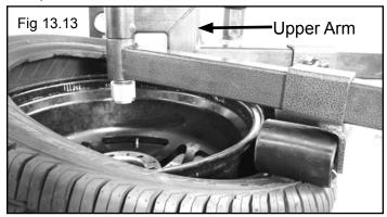
10. Depress the Table Top Pedal. As the Turntable rotates the Lower Arm will follow the tire around. Keep rotating the table until the bead is mounted. (See Fig 13.14 - 13.16)
