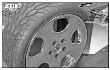
7. Turn wheel around and repeat procedure on the other side of the wheel. This should be the long side of the drop center. It will be easier to clamp the wheel to the table top if the lower bead is loosened last. (See Fig. 11.4)
