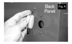
Insert the circular foam filter into the recess in the Air Vent Cover, and attach the cover to the rear of the cabinet as shown in Fig.4, having first pried out the plastic bung from the vent hole.
