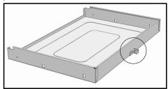
**NOTE:** If the drawer was slammed while the locking mechanism was engaged, and damage to the mechanism is suspected, follow instructions provided in this manual to remove the drawer. Inspect the locking tab for damage. Use a screwdriver to straighten the tab.
